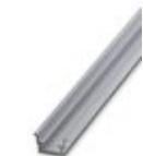
DIN rail, unperforated, Standard profile, width: 35 mm, height: 15 mm, similar to EN 60715, material: Aluminum, uncoated, length: 2000 mm, color: silver
